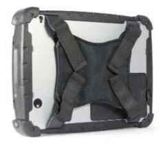
On the back, the Duros has a handstrap with four elastic Velcro strips to adjust the strap to your hand. Should it break, or you do not want it for a deployment, remove it by undoing four Philips screws.
