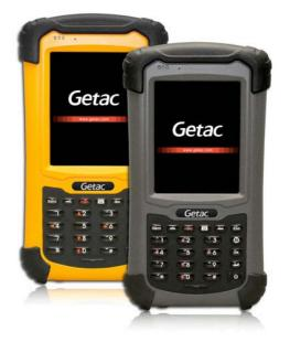
802.11b/g WiFi. A SIM slot, located inside the battery compartment, enables the unit to function as a phone and also enables HSDPA wireless WAN communication (Getac offers a special HSDPA model of the PS236). Wired connectivity includes serial and USB 2.0.
