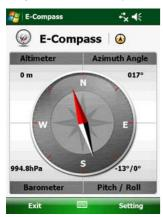
is enough for most mapping and GPS applications. Post processing can result in even better accuracy, down to the sub-meter range. The PS236 includes a separate altimeter and can determine pitch and roll. It can also detect barometric pressure. There
